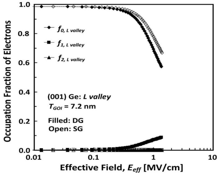
Fig. 7. Simulated occupation fractions ( $f_0$ ,  $f_1$  and  $f_2$ ) of electrons sharing the lowest and higher subbands as a function of  $E_{eff}$  for the  $L$  valley at  $T_{GOI}$  of 7.2 nm where (001) Ge surface is assumed.
