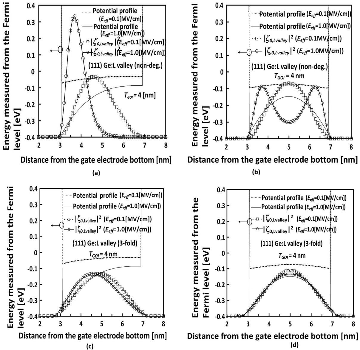
Fig. 21. Simulated profiles of wave functions of electrons sharing the non-degenerate and 3-fold  $L$  valleys for SG and DG GOI MOSFETs with (111) Ge surface channel for two different  $E_{eff}$  values at  $T_{GOI}$  of 4 nm: a) electrons sharing the non-degenerate  $L$  valley of SG MOSFET; b) electrons sharing the non-degenerate  $L$  valley of DG MOSFET; c) electrons sharing the 3-fold  $L$  valley of SG MOSFET; d) electrons sharing the 3-fold  $L$  valley of DG MOSFET.
