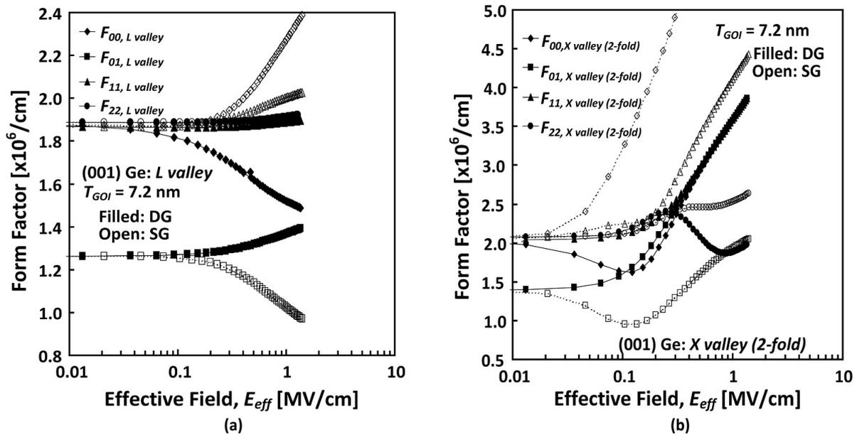
Fig. 10. Simulated form factors ( $F_{ij}$ ) of electrons sharing the lowest, 1<sup>st</sup> and 2<sup>nd</sup> excited subbands of the *L* or *X* valley as a function of  $E_{eff}$  for SG and DG GOI MOSFETs with (001) Ge surface channel at  $T_{GOI} = 7.2$  nm: a) *L* valley; b) 2-fold *X* valley.
