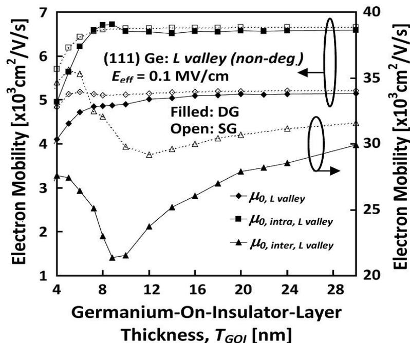
Fig. 17. Simulated phonon-limited mobility of electrons sharing the lowest subband of the non-degenerate  $L$  valley on the (111) Ge surface as a function of  $T_{GOI}$  at  $E_{eff} = 0.1$  MV/cm.  $\mu_{0,intra,Lvalley}$  and  $\mu_{0,inter,Lvalley}$  are also shown separately.
