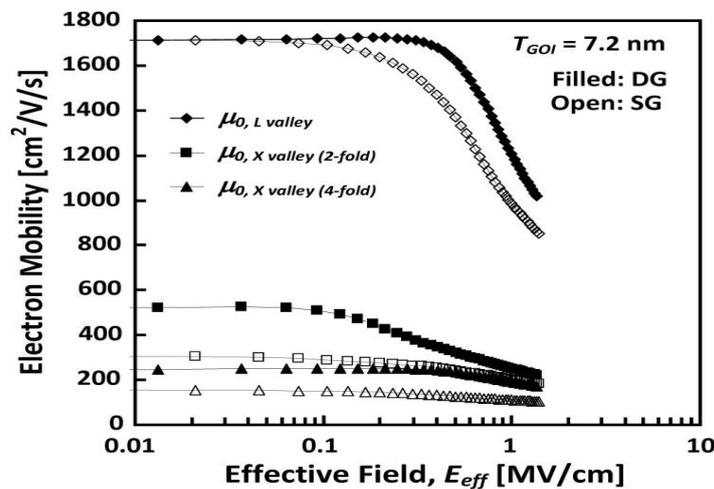
Fig. 6. Simulated phonon-limited mobility of electrons sharing the lowest subband of  $L$  or  $X$  valley on the (001) Ge surface as a function of  $E_{eff}$  at  $T_{GOI}$  of 7.2 nm.
