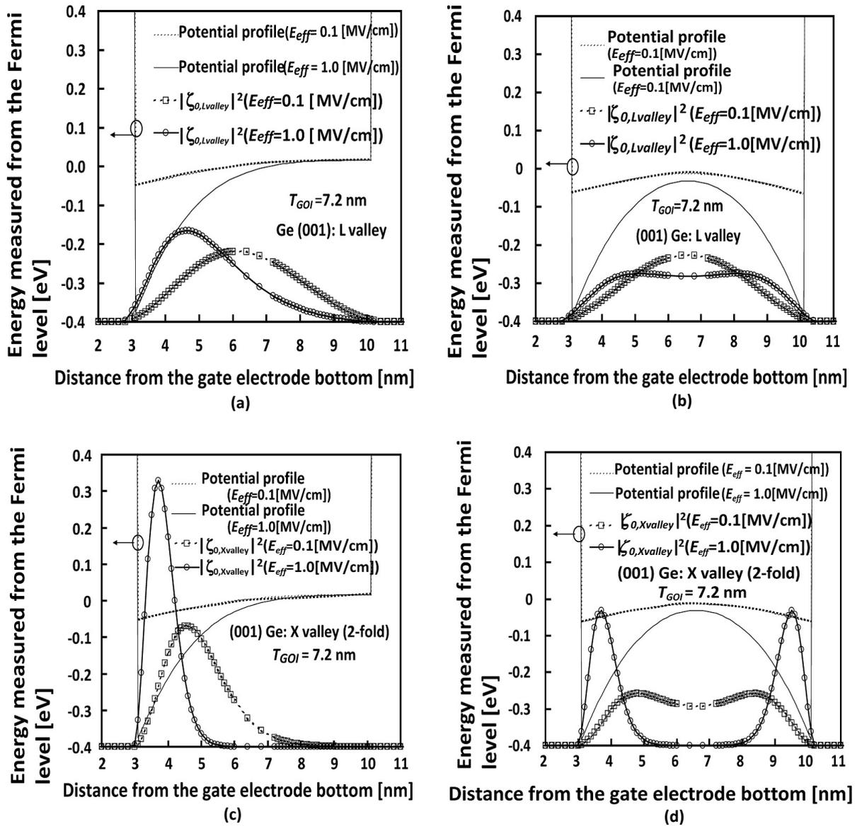
Fig. 12. Simulated profiles of wave functions of electrons sharing the  $L$  valley and 2-fold  $X$  valleys for SG and DG GOI MOSFETs with (001) Ge surface channel for two different  $E_{eff}$  values at  $T_{GOI}$  of 7.2 nm: a) electrons sharing the  $L$  valley of SG MOSFET; b) electrons sharing the  $L$  valley of DG MOSFET; c) electrons sharing the 2-fold  $X$  valley of SG MOSFET; d) electrons sharing the 2-fold  $X$  valley of DG MOSFET.
