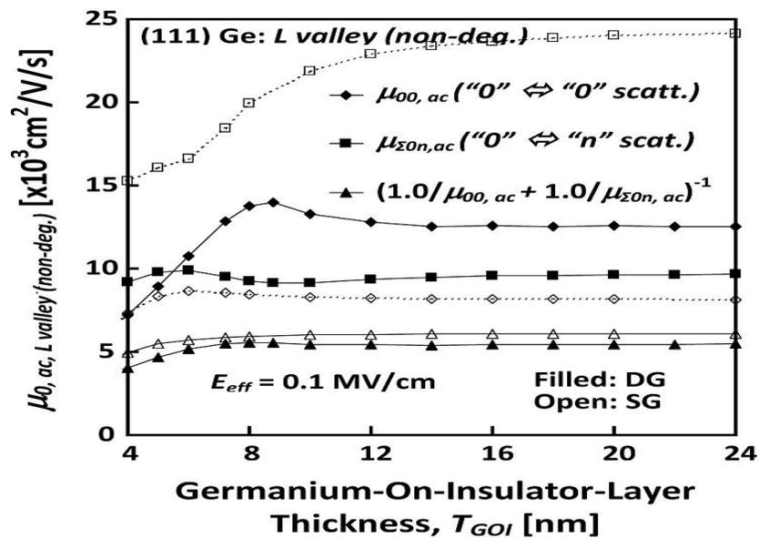
Fig. 20. Simulated acoustic-phonon-limited mobility of electrons sharing the non-degenerate  $L$  valley on the (111) Ge surface as a function of  $T_{GOI}$  at  $E_{eff} = 0.1$  MV/cm. Components of acoustic-phonon-scattering-limited mobility are shown separately.
