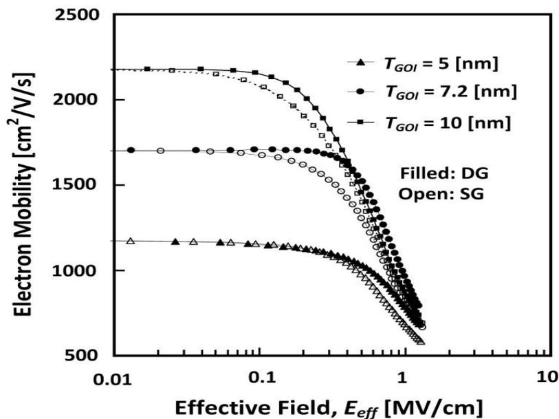
Fig. 3. Simulated phonon-limited electron mobility on the (001) Ge surface as a function of  $E_{eff}$  for DG and SG GOI MOSFETs; the parameter is the GOI layer thickness.
