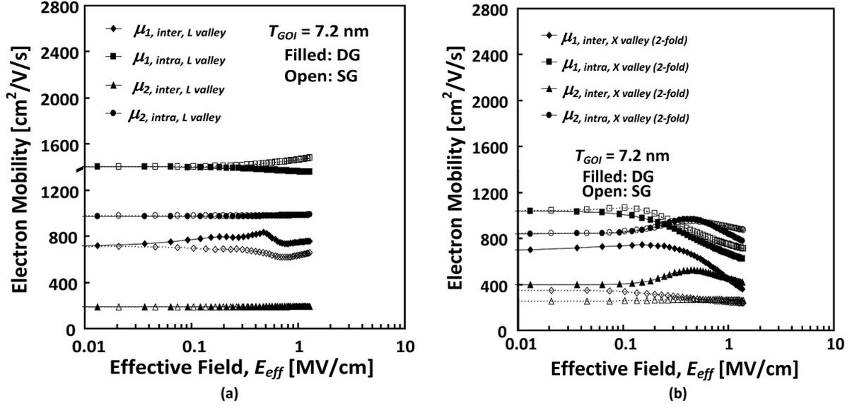
Fig. 9. Intra-valley-phonon-scattering-limited mobility ( $\mu_{0, \text{intra}}$ ), inter-valley-phonon-scattering-limited mobility ( $\mu_{0, \text{inter}}$ ), and overall phonon-limited mobility of electrons sharing the 1<sup>st</sup> and 2<sup>nd</sup> excited subbands of the L or X valley as a function of  $E_{\text{eff}}$  for SG and DG GOI MOSFETs with (001) Ge surface channel at  $T_{\text{GOI}} = 7.2 \text{ nm}$ : a) L valley; b) 2-fold X valley.
