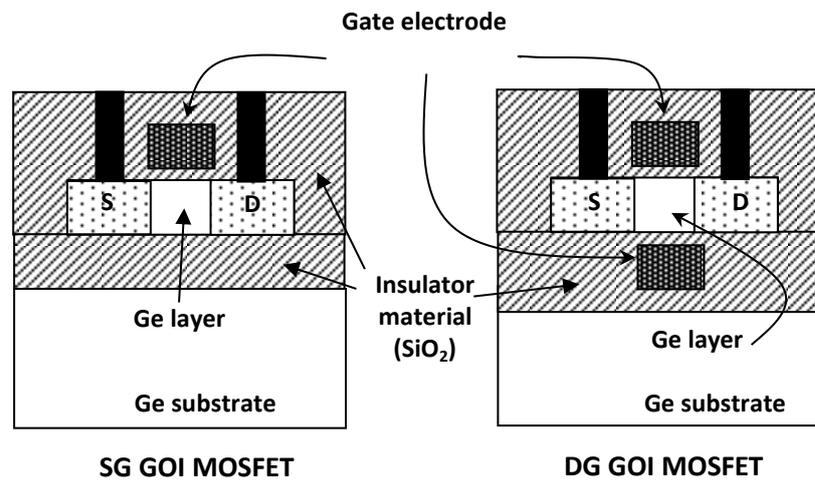
Fig. 1. Simplified cross-sectional views of SG and DG GOI MOSFETs where 'S' denotes the source diffusion region, and 'D' denotes the drain diffusion region.
