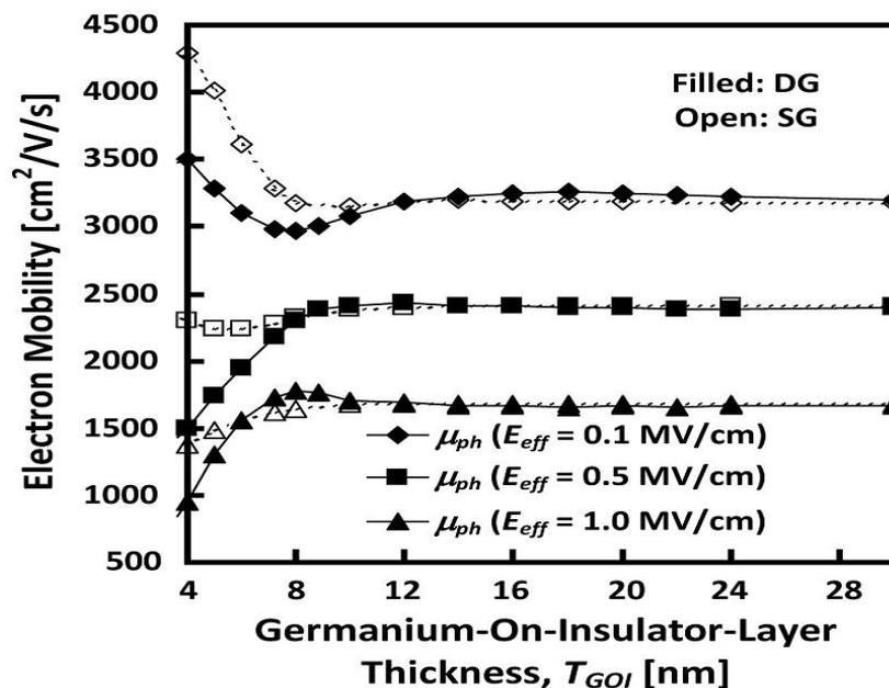
Fig. 13. Simulated phonon-limited electron mobility on the (111) Ge surface as a function of  $T_{GOI}$  for various  $E_{eff}$  values; simulated mobility values of the DG and SG GOI MOSFETs are compared.
