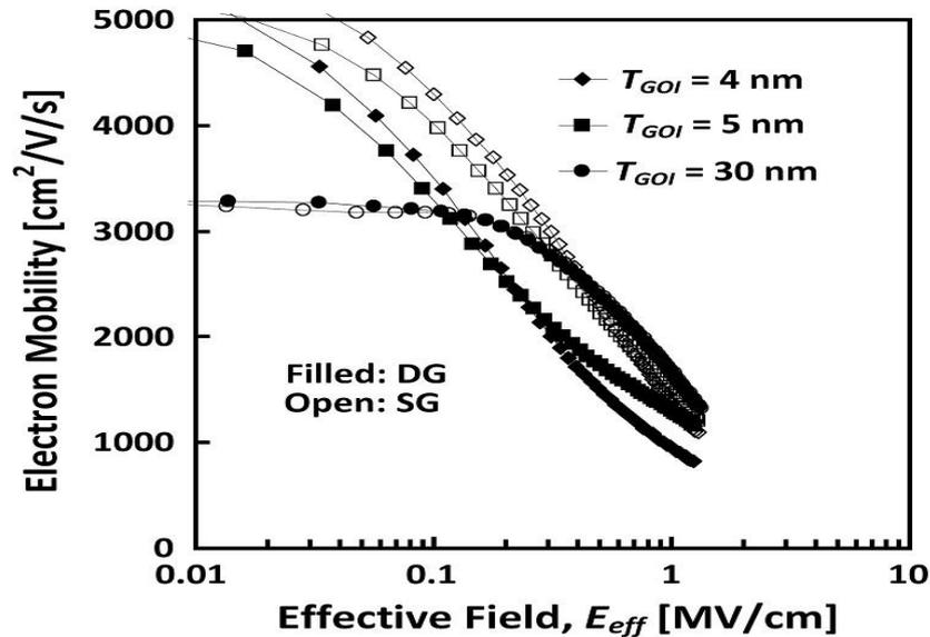
Fig. 14. Simulated phonon-limited electron mobility on the (111) Ge surface as a function of  $E_{eff}$  for DG and SG GOI MOSFETs; the parameter is GOI layer thickness.
