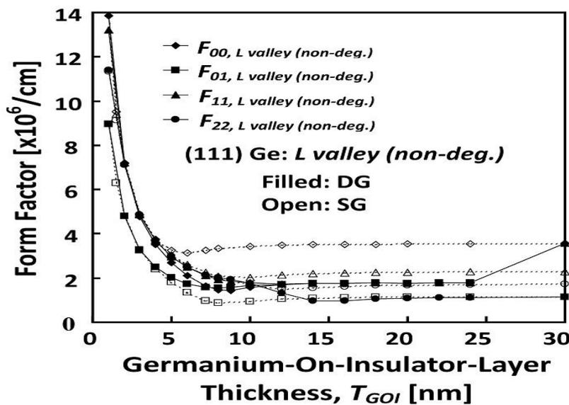
Fig. 19. Simulated form factors ( $F_{ij}$ ) of electrons sharing the non-degenerate  $L$  valley as a function of  $T_{GOI}$  for SG and DG GOI MOSFETs with (111) Ge surface channel.
