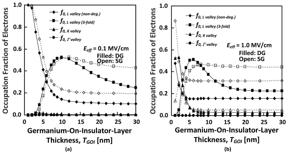
Fig. 16. Simulated occupation fractions of electrons sharing the lowest subband as a function of  $T_{GOI}$  for  $L$  (non-degenerate and 3-fold),  $X$  and  $\Gamma$  valleys on the (111) Ge surface: a) low-field condition ( $E_{eff} = 0.1$  MV/cm); b) high-field condition ( $E_{eff} = 1$  MV/cm).
