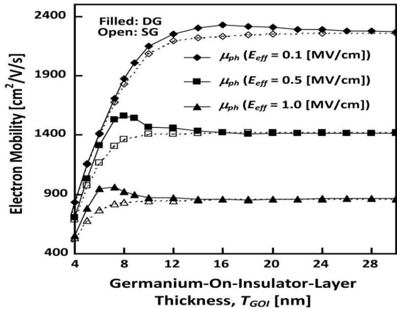
Fig. 2. Simulated phonon-limited electron mobility on the (001) Ge surface as a function of  $T_{GOI}$  for various  $E_{eff}$  values; simulated mobility values of DG and SG GOI MOSFETs are compared.
