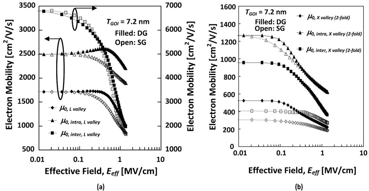
Fig. 8. Intra-valley-phonon-scattering-limited mobility ( $\mu_{0, intra}$ ), inter-valley-phonon-scattering-limited mobility ( $\mu_{0, inter}$ ), and overall phonon-limited mobility of electrons sharing the lowest subband of the  $L$  or  $X$  valley as a function of  $E_{eff}$  for SG and DG GOI MOSFETs with (001) Ge surface channel for  $T_{GOI} = 7.2$  nm: a)  $L$  valley; b) 2-fold  $X$  valley.
