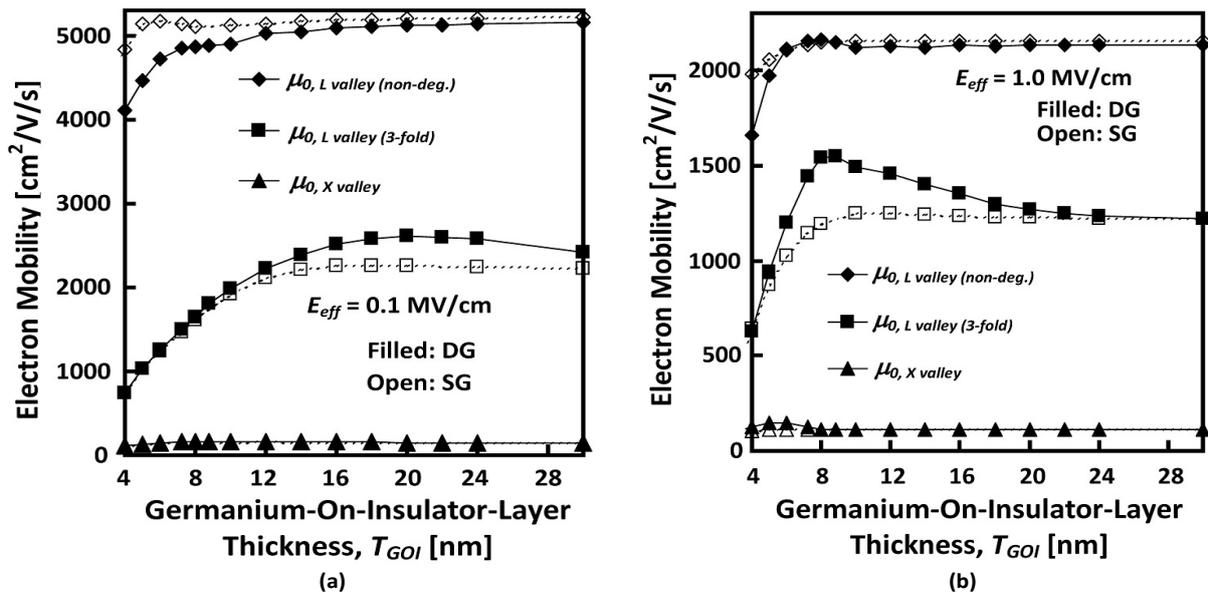
Fig. 15. Simulated phonon-limited mobility of electrons sharing the lowest subband as a function of GOI-layer thickness ( $T_{GOI}$ ) for  $L$  (non-degenerate and 3-fold) and  $X$  valleys where (111) Ge surface is assumed: a) low-field condition ( $E_{eff} = 0.1$  MV/cm); b) high-field condition ( $E_{eff} = 1$  MV/cm).
