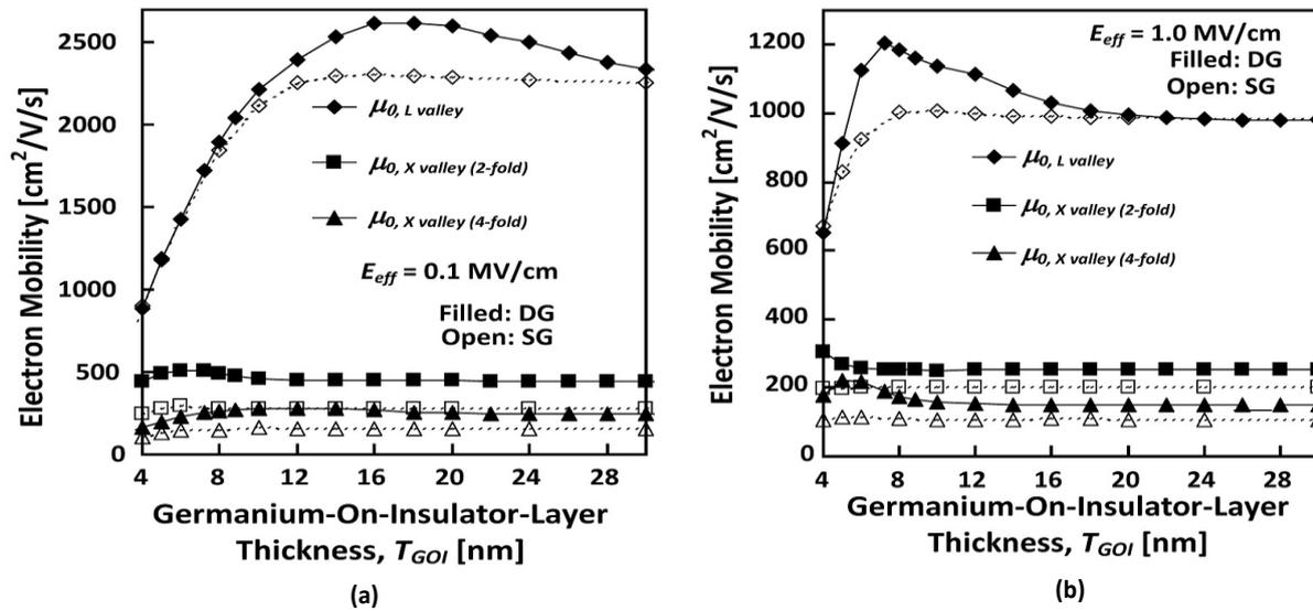
Fig. 5. Simulated phonon-limited mobility of electrons sharing the lowest subband of  $L$  or  $X$  valley on the (001) Ge surface as a function of  $T_{GOI}$  for various  $E_{eff}$  values: a) low-field condition ( $E_{eff} = 0.1$  MV/cm); b) high-field condition ( $E_{eff} = 1$  MV/cm).
