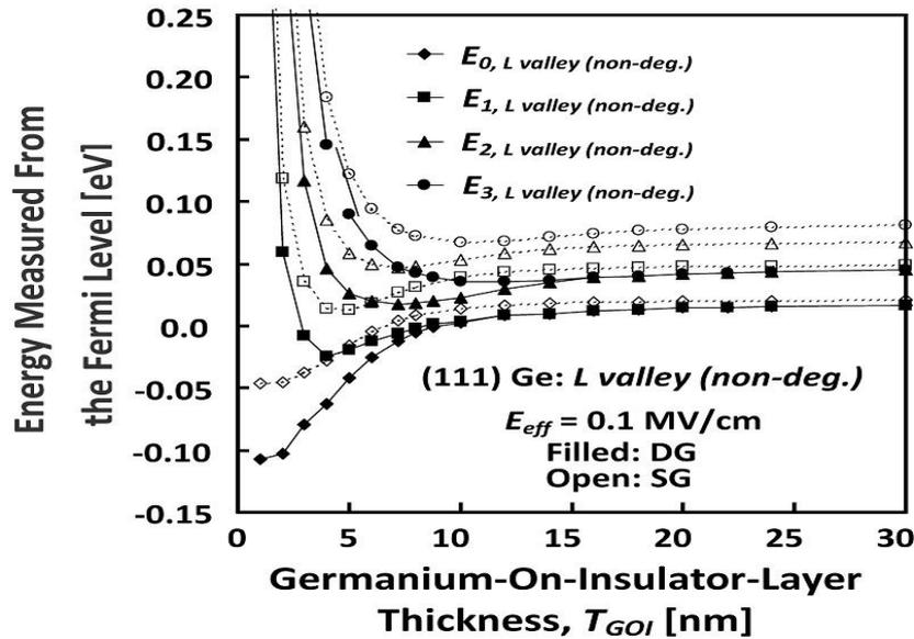
Fig. 18. Simulated subband energy levels ( $E_0$ ,  $E_1$ ,  $E_2$ , and  $E_3$ ) measured from the Fermi level as a function of  $T_{GOI}$  in the  $L$  valley on the (111) Ge surface at  $E_{eff} = 0.1$  MV/cm.
