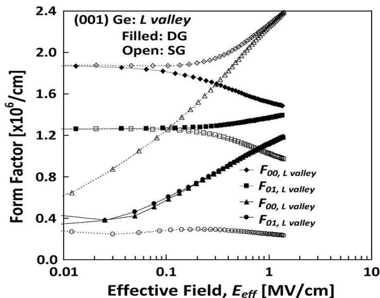
Fig. 11. Simulated form factors ( $F_{ij}$ ) of electrons sharing the lowest and 1<sup>st</sup> excited subbands of the *L* or *X* valley as a function of  $E_{eff}$  for SG and DG GOI MOSFETs with (001) Ge surface channel for two different  $T_{GOI}$  values.
