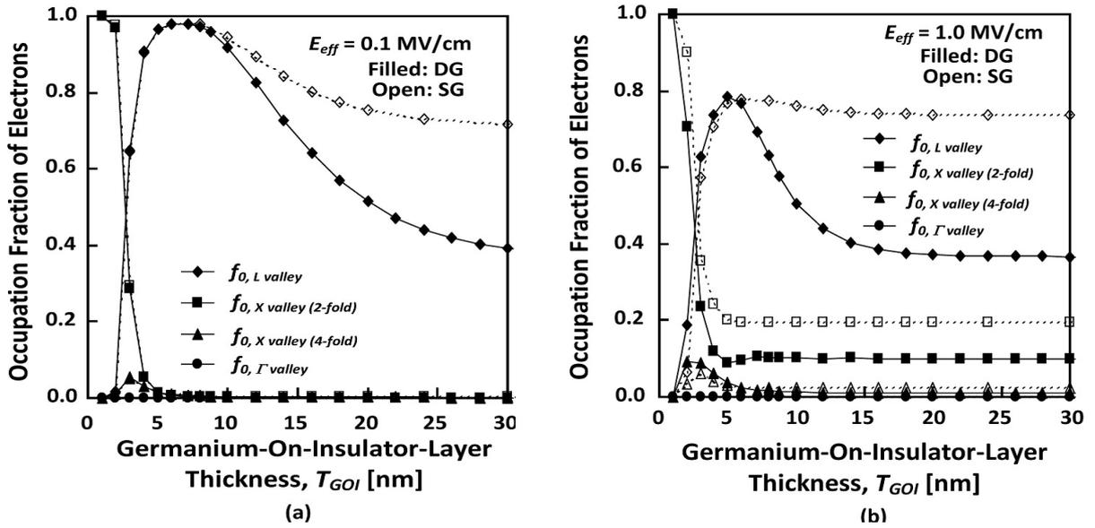
Fig. 4. Occupation fraction of electrons in lowest subband as a function of GOI-layer thickness ( $T_{GOI}$ ) for  $L$ ,  $X$  (2-fold and 4-fold) and  $\Gamma$  valleys where (001) Ge surface is assumed: a) low-field condition ( $E_{eff} = 0.1$  MV/cm); b) high-field condition ( $E_{eff} = 1$  MV/cm).
